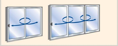
Versi-Panel doors are completely reversible during installation. Doors can be easily configured for left- or right-hand operation. Choice of two, three or four-panel (non-reversible) models in a range of standard sizes (custom sizes available).
