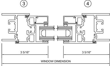
\*FRAMING SHOWN AS EQUAL LEG, ALSO AVAILABLE IN NAIL FIN, FLANGE FRAME AND PROJECT SPECIFIC APPLICATIONS.
