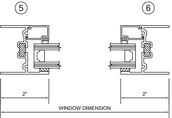
\*FRAMING SHOWN AS EQUAL LEG, ALSO AVAILABLE ARE NAIL FIN, FLANGE FRAME, AND PROJECT SPECIFIC APPLICATIONS.
