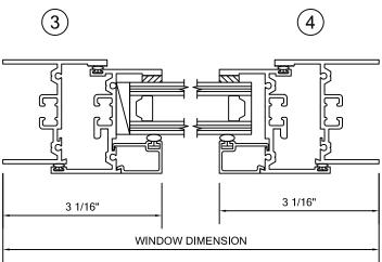
\*FRAMING SHOWN AS EQUAL LEG, ALSO AVAILABLE IN NAIL FIN, FLANGE FRAME AND PROJECT SPECIFIC APPLICATIONS.
