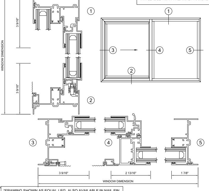
\*FRAMING SHOWN AS EQUAL LEG, ALSO AVAILABLE IN NAIL FIN, FLANGE FRAME AND PROJECT SPECIFIC APPLICATIONS.
